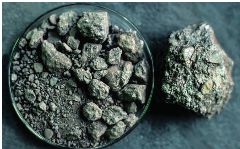
Fig. 6. A pair of fist-sized specimens of the Vasquez Conglomerate were collected in 1979 from the hillside where the St Francis Dam had once stood. One specimen was then placed in a beaker of water for 15 minutes, before being drained and dried, by which time it had completely fallen apart.
